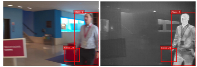
Fig. 3: Sample frame with RGB to thermal label transfer
